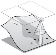
Sonar is very fast. A sound wave can travel from the surface to a depth of 240' (70m) and back again in less than 1/10 of a second. It is unlikely that your boat can "outrun" this sonar signal.
